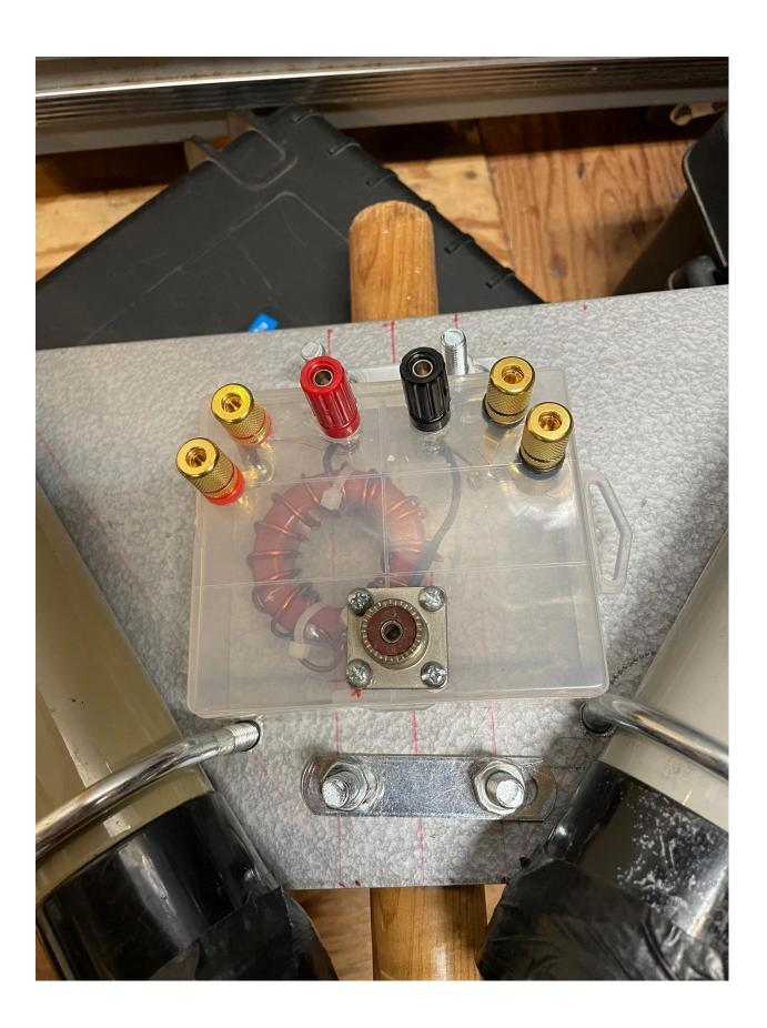
The toroid used is T130-2 and the magnet wire is AWG18 size.
